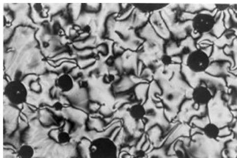
FIGURE 7 Smectic C schlieren texture of 6–12 at 236°C.
