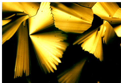
Figure 1a. Optical textures of compound 4 at 68.6\text{ }^\circ\text{C} , in a polyimide-coated thin-cell with a cell gap of d = 5 \pm 0.2\text{ }\mu\text{m} with homogeneous planar boundary conditions.
