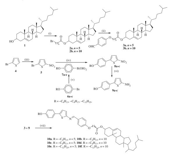
Scheme 1. Reagents and conditions: (i) bromoalkanoyl chloride, tetrahydrofuran (THF), pyridine, room temperature (rt), (ii) p-hydroxy benzaldehyde, acetone,  $K_2CO_3$ , reflux, (iii) HNO<sub>3</sub>, acetic anhydride, icebath, (iv) Pd(PPh<sub>3</sub>)4, 2.0 M aq. Na<sub>2</sub>CO<sub>3</sub>, (v) n-BuLi, B(OMe)<sub>3</sub>, THF, -78°C rt, (vi) H<sub>2</sub>, Pd/C, rt, (vii) dry alcohol, acetic acid (cat), reflux.
