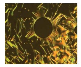
Figure 3. The Cholesteric–TGB–SmA transition of compound **10c** at 179°C (colour version online).
