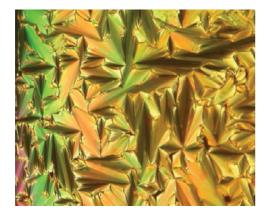
Figure 4. The texture of compound 10c at  $175^{\circ}C$  (colour version online).
