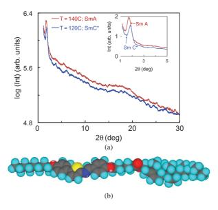
Figure 6. (a) XRD diagram of compound **10c** in the SmA and SmC phases. The inset shows the low angle reflections on an enlarged scale. (b) Energy minimised configuration of the molecule **10c** obtained using the MM2 package (colour version online).
